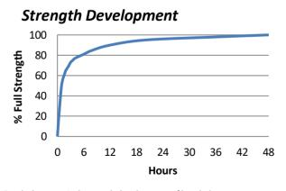
Graph shows typical strength development of bonded components at 23°C. Curing at higher or lower temperatures may affect cure speed.
